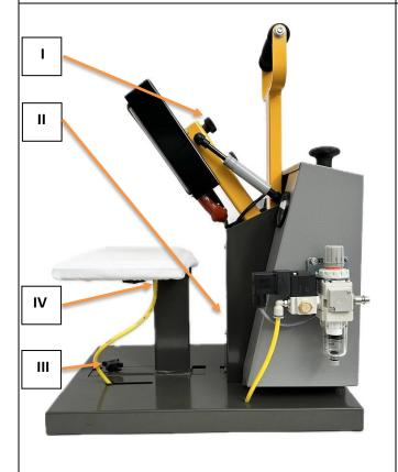
Place the heated plate onto the lever and fix it with the fastening screw marked by number "I".
