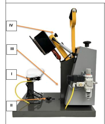
Please unplug the air tube marked by "I". - You can pull the air tube out by pushing the ring at the end of the air connector in the direction of the connector.
